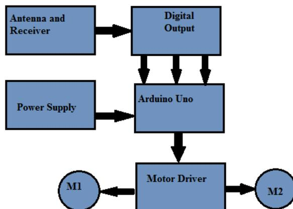
Fig: 2- Block diagram of receiver module
