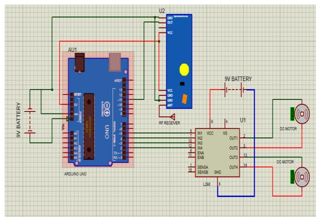
Fig. 4: Circuit diagram of the receiver section
