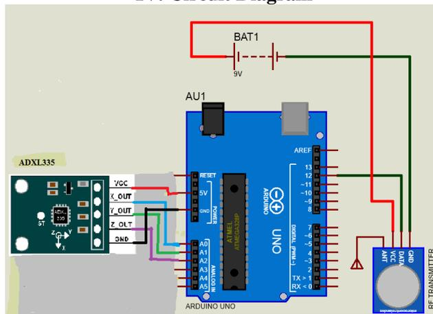
Fig. 3: Circuit diagram of the transmitter section.
