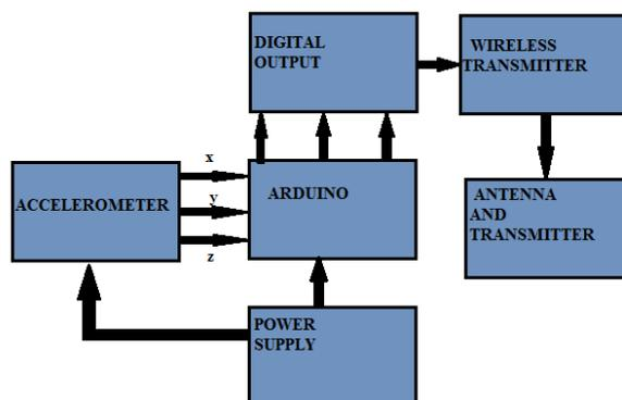
Fig: 1. Block diagram of transmitter module
